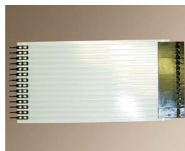
FFC254 + HOUSING + MALE PIN
